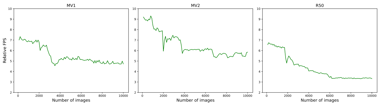
FIGURE 16. Throughput variations over 100 image intervals for processing 10,000 images on Pixel 6.
