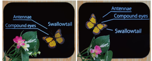
FIGURE 13. Annotations of mid-air images are displayed at positions that do not overlap with the shape of real objects obtained from the depth sensor.
