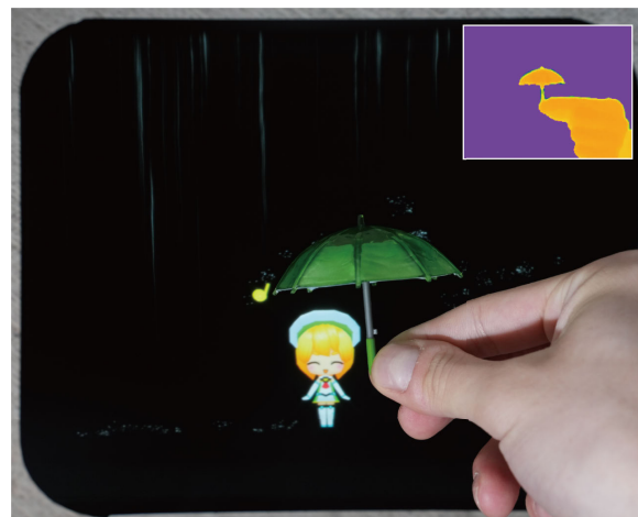
FIGURE 10. In our system, a miniature umbrella is used to protect the character displayed as a mid-air image from getting wet in the rain. The picture-in-picture image shows that a depth camera can capture the shape of real objects.
