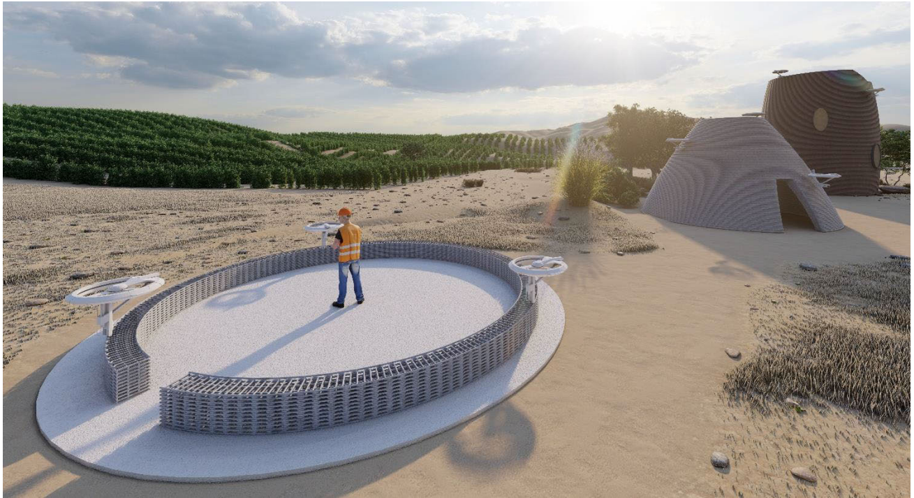
FIGURE 1. The conceptual representation of aerial additive building manufacturing (AAM) with multiple coordinated unmanned aerial vehicles (UAV) extruding a suitable pseudoplastic mortar in a customised continuous curve printing path.
