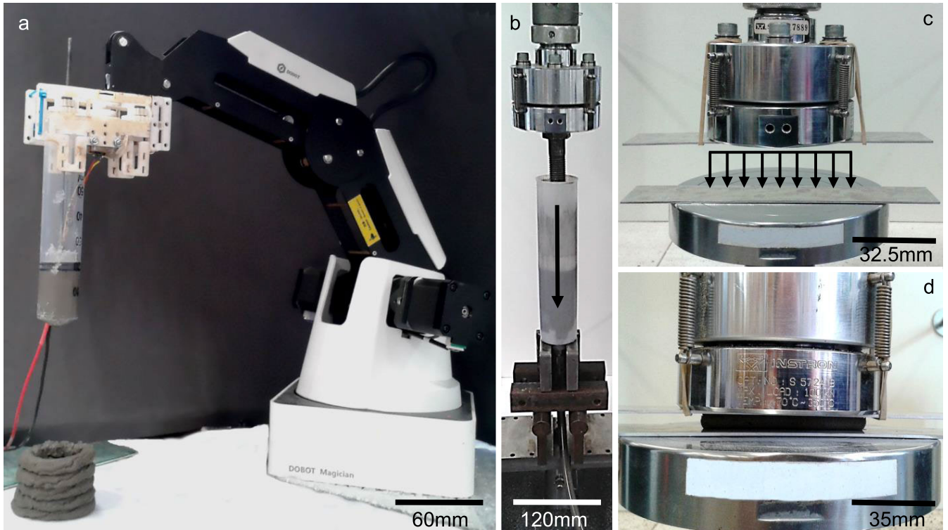
FIGURE 5. Robotic arm, axial force and material deformation tests. a) Robotic arm manipulating a 60 ml capacity device printing a fresh mix. b) Axial force test rig with direction of force indicated. c,d) Material deformation test rig shown with direction of uniformly distributed load indicated (c) and evaluating the settlement of an 8 mm diameter bead of extruded fresh material (d).
