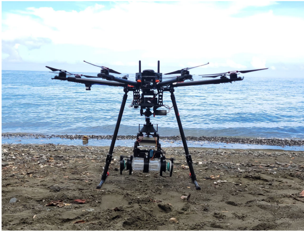
FIGURE 1. Actual image of drone-based automatic water sampling system.
