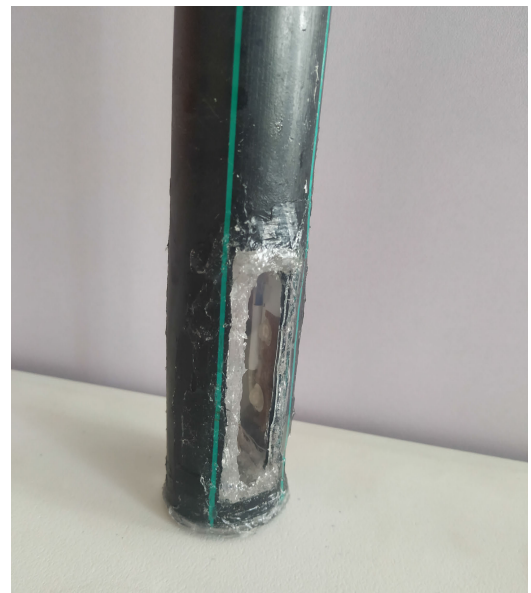
FIGURE 6. Housing zone designated for absorbance sensor placement.
