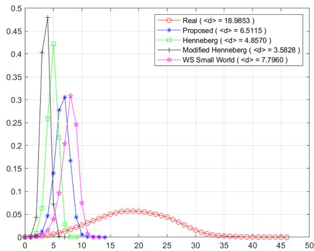
**FIGURE 15.** Distance Distribution of the real dataset (US Western States Power Grid), the proposed model, Henneberg’s Model, Modified Henneberg’s Model, and WS Small World Model. The legend in the graph shows the average path length of each network.
