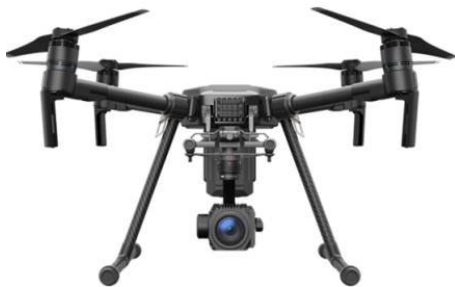
FIGURE 20. M200 drone with an onboard Z30 PTZ camera [107].
