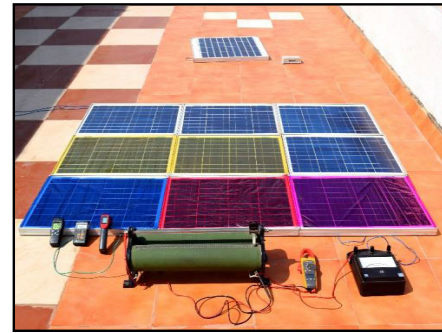
FIGURE 13. Experimental setup of a 3 \times 3 PV array.
