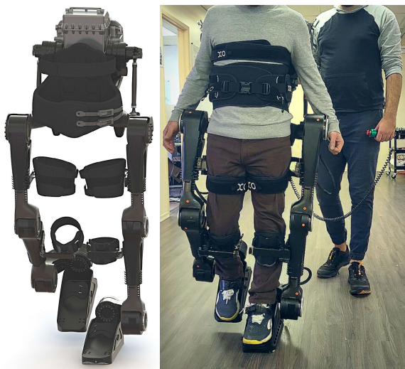
FIGURE 1. Human subject wearing the XoMotion Beta 2 exoskeleton used in this work (Human in Motion Robotics Inc., Vancouver, BC).
