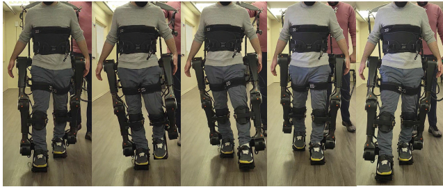
FIGURE 3. Snapshots of a test user walking with the XOMotion Beta 2 exoskeleton, using predicted walking parameters from GPR (the sequence is from left to right taking two steps).
