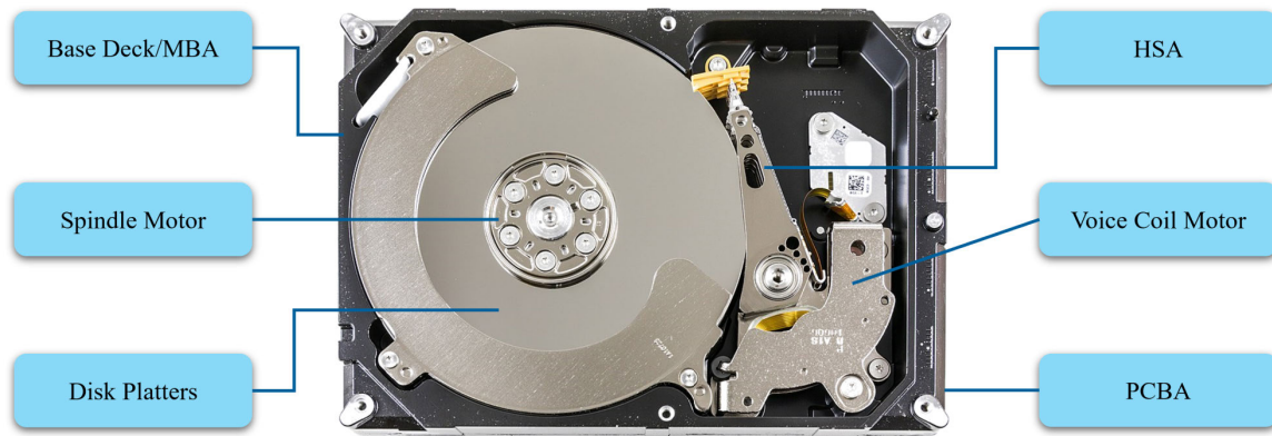
FIGURE 4. A diagram of the hard disk drive components, showing the base deck, spindle motor, disk platters, head stack assembly, voice coil motor, and printed circuit board assembly.
