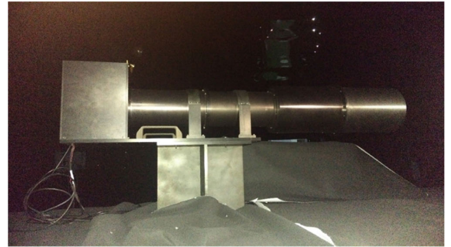
FIGURE 12. Physical drawing of calibration lens (including hood) after installation and adjustment.
