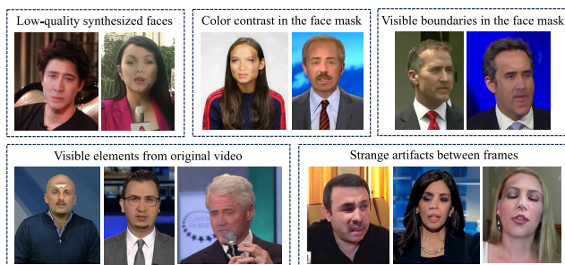
FIGURE 5. Artifacts and weaknesses in fake images that limit their naturalness and facilitate fake detection [31].
