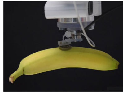
FIGURE 6. Suction cup manufactured in flexible resin using DLS technology [44].
