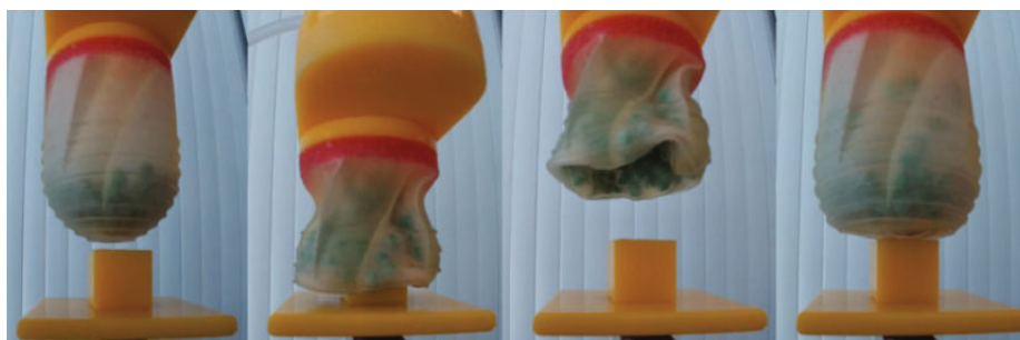
FIGURE 5. 3D printed jamming gripper manufactured in a one-shot configuration using PolyJet technology [33].
