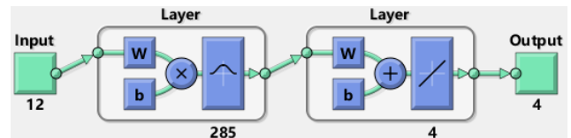
FIGURE 8. Neural network framework. According to the evaluation system, the data samples were used to build a training network. The dimension of the input signal refers to the number of secondary indexes.
