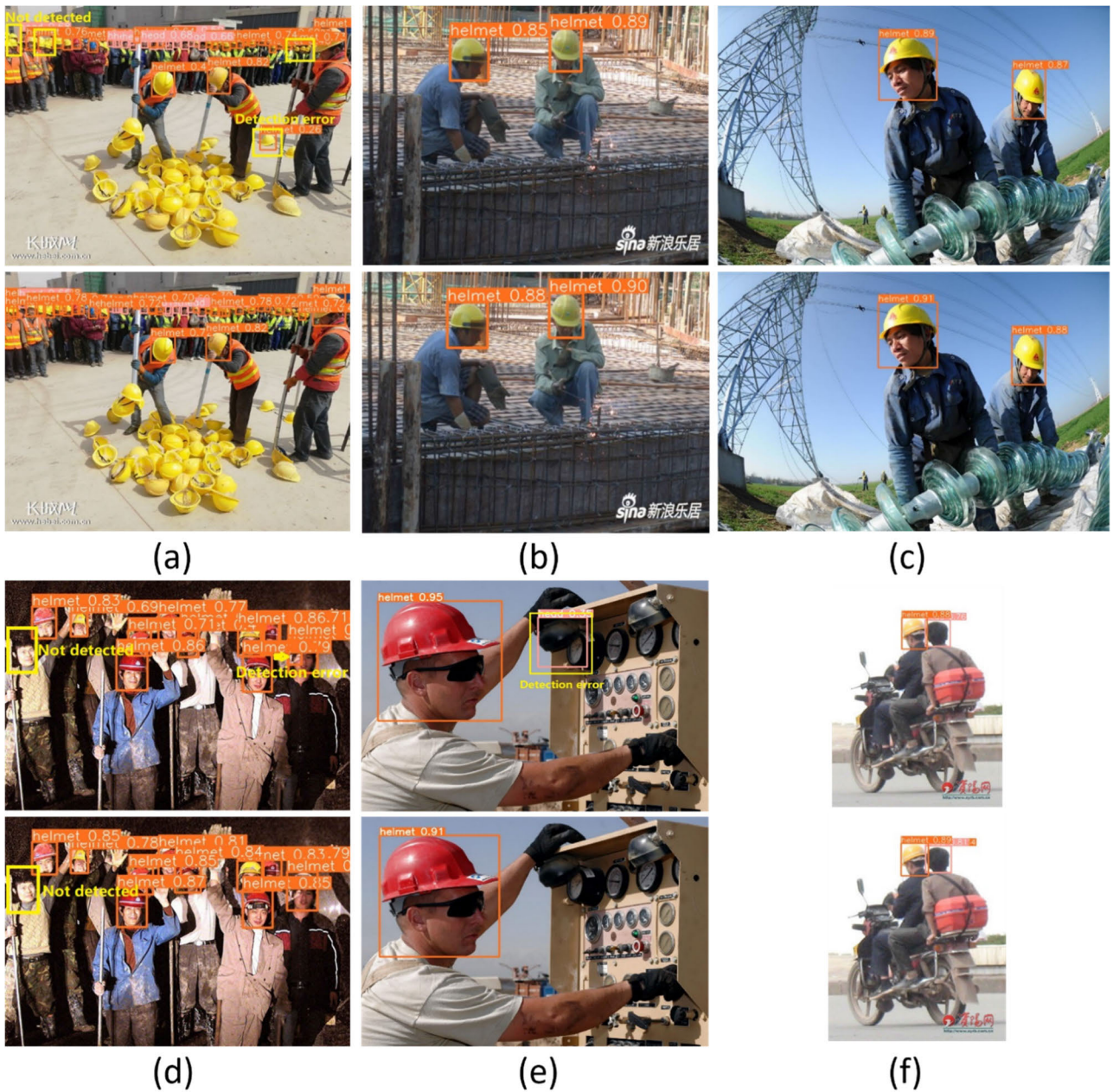
FIGURE 14. Comparison of the detection performance in various real-world application scenarios between YOLOv8n and YOLOv8n-SLIM-CA (the first row represents the detection results of YOLOv8, and the second row represents the detection results of YOLOv8n-SLIM-CA). (a) Open outdoor spaces; (b) Construction sites; (c) The power industry; (d) Mines; (e) Engineering operations; (f) Traffic safety.
