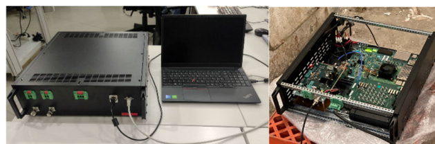
FIGURE 12. BPL prototypes during laboratory tests (left) and real deployment (right).
