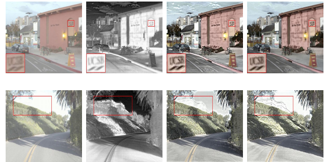
FIGURE 14. Ablation results corresponding to different network structures. The first and second columns represent visible and infrared images respectively, while the third and fourth columns represent fusion results without ECB processing and fusion results using our method respectively.
