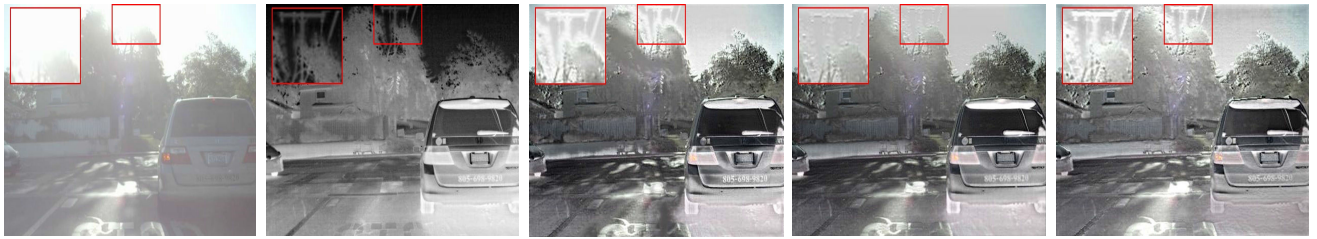
FIGURE 12. Representative examples of ablation results under different parameters. The first and second columns are infrared and visible images respectively, while the last three columns are subjective ablation results with hyperparameters \alpha = 10, \beta = 1, \alpha = 1, \beta = 10 and \alpha = 1, \beta = 1 respectively.
