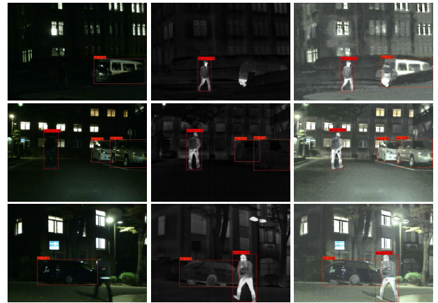
FIGURE 15. Results of object detection. (Top to bottom) 00689N, 01042N, and 00054N. (Left to right) visible images, infrared images and fused images of our method, respectively.
