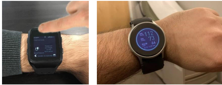
a) Blood pressure smartwatch using optical sensor [30] b) Blood pressure smartwatch comes with inflatable strap [58]
