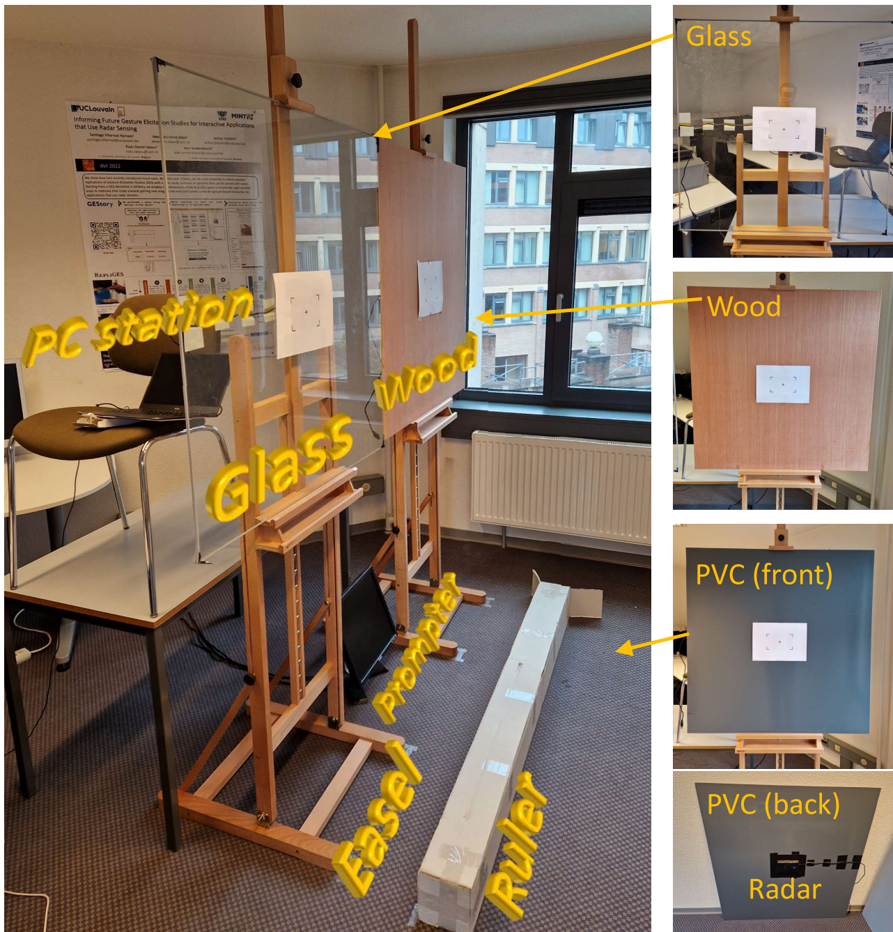
FIGURE 6. Setup for radar-based gesture acquisition through three materials: wood, glass, and PVC.
