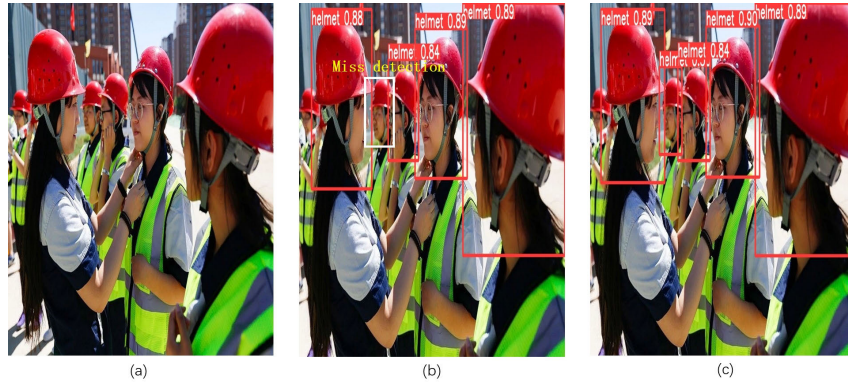
FIGURE 13. Comparison of detection before and after Soft-NMS improvement: (a) Image, (b) YOLOv5n detection results, (c) Soft-NMS detection results.
