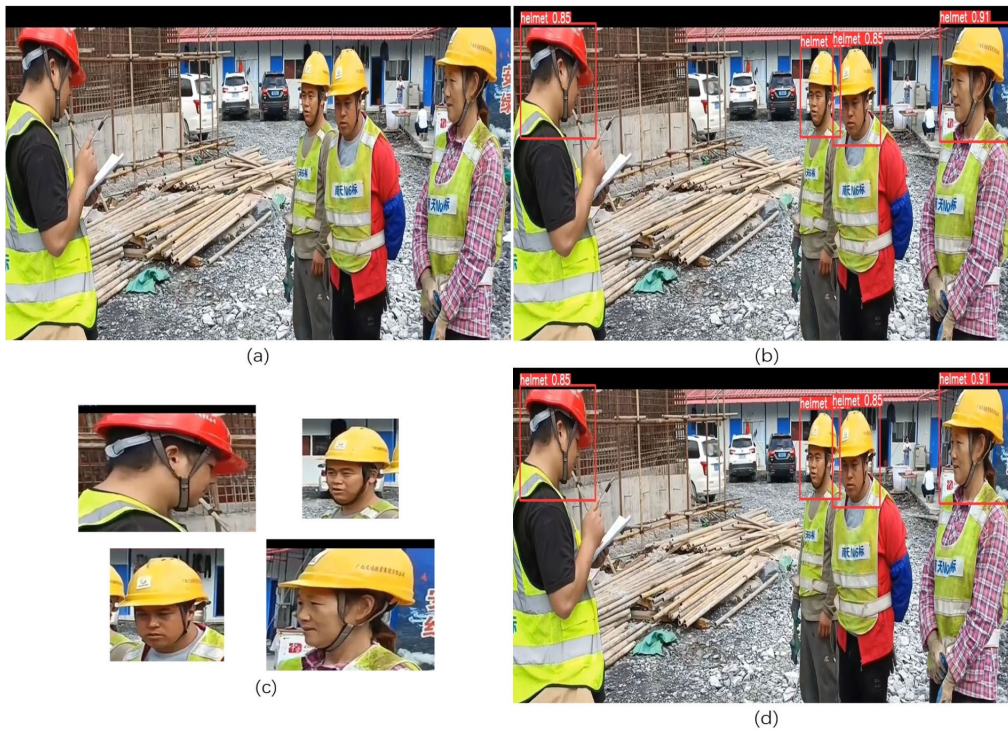
FIGURE 6. Automatic storage function renderings: (a) Video-captured image, (b) detection result, (c) original YOLOv5n capture function, and (d) YOLO-ESCA automatic savings function.
