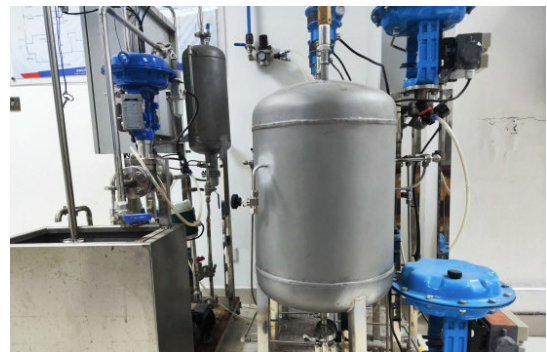
FIGURE 13. Equipment diagram for temperature-pressure control.
