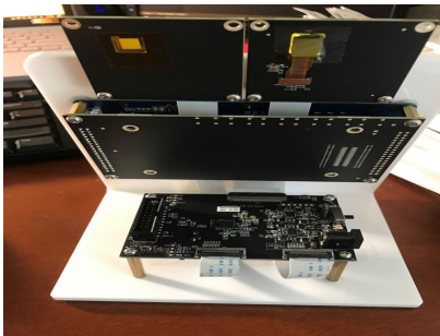
FIGURE 6. Kneron KL520 hardware assembly.
