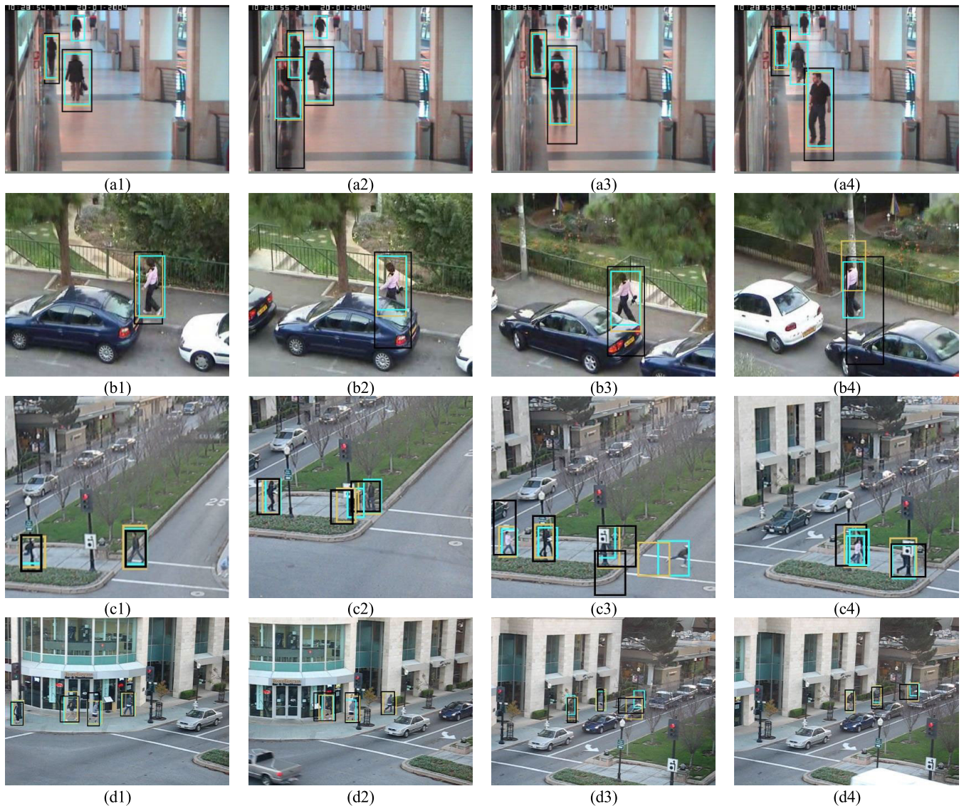
FIGURE 7. Comparison of tracking effects. For clarity of display, only KCF, ECO and the algorithm C-ECO are used in this paper. black boxes are KCF, yellow boxes are ECO and blue boxes are C-ECO.
