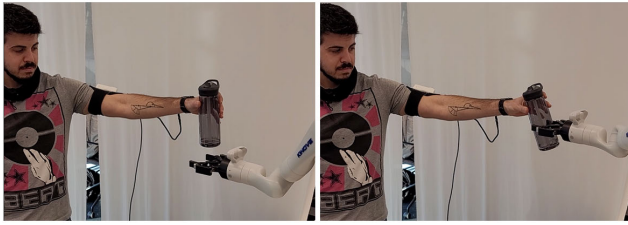
FIGURE 13. An HRC demonstration in which participant 1 hands-over a bottle to the robot.
