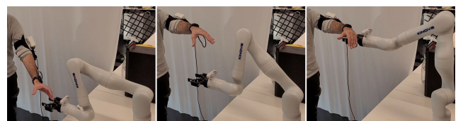
FIGURE 12. Motion of participant 2 between two arm poses within the interaction space while the robotic arm follows.
