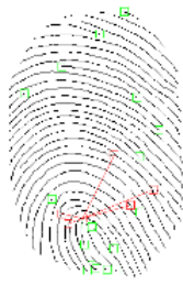
(a) constructing the feature point description operator through the intersection points of fingerprint secondary features
