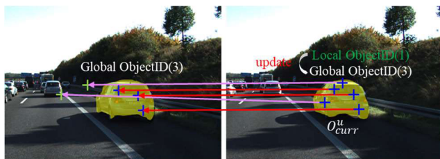
FIGURE 5. Description of Object Level Tracking. Left: ObjectID is assigned to features in the previous frame. Right: Local features in the current frame is matched with the global ObjectID features.
