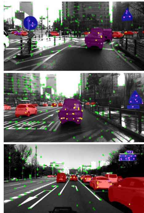
FIGURE 9. Examples of detecting traffic sign features. There are multiple image features on various traffic signs.
