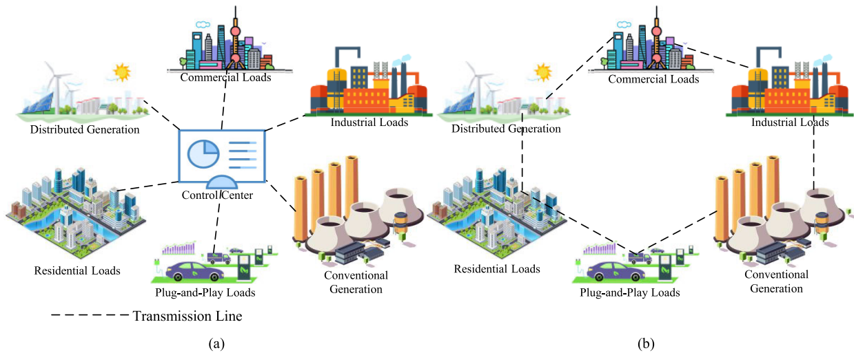
FIGURE 1. Different approaches for power grids. (a) centralized approach; (b) decentralized approach (bus-to-bus).
