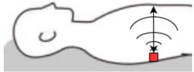
FIGURE 10. Placement of the ultrasound sensor to obtain ground truth from a CPR Manikin. The torso outline represents the Manikin, while the red box illustrates the location of the sensor measuring the distance indicated by the arrow.
