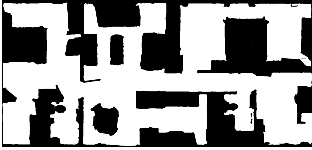
FIGURE 3. Visualization of the Cantwell environment, where the black regions represent unfeasible areas and the white regions represent feasible areas.
