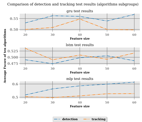
FIGURE 22. Comparison of detection and tracking results: average values for the 10 best feature selection algorithms.
