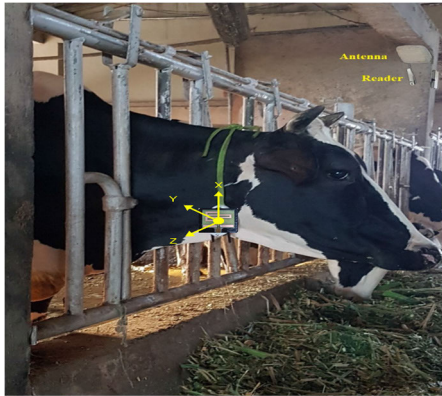
FIGURE 8. Sensor mounted on the cow’s neck and the position of the reader.
