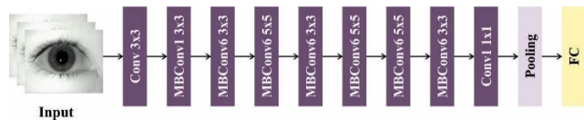
FIGURE 2. Architecture of the EfficientNet model.
