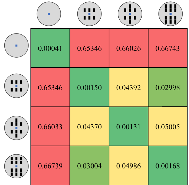
FIGURE 12. Heatmap of the dissimilarity score for various scenarios containing different number of vehicles in the scene. The occlusion from 12 cars scene, causes the similarity score to decrease.
