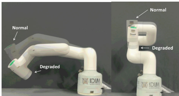
FIGURE 8. Movement results of normal and degraded robot manipulator for the same target point.
