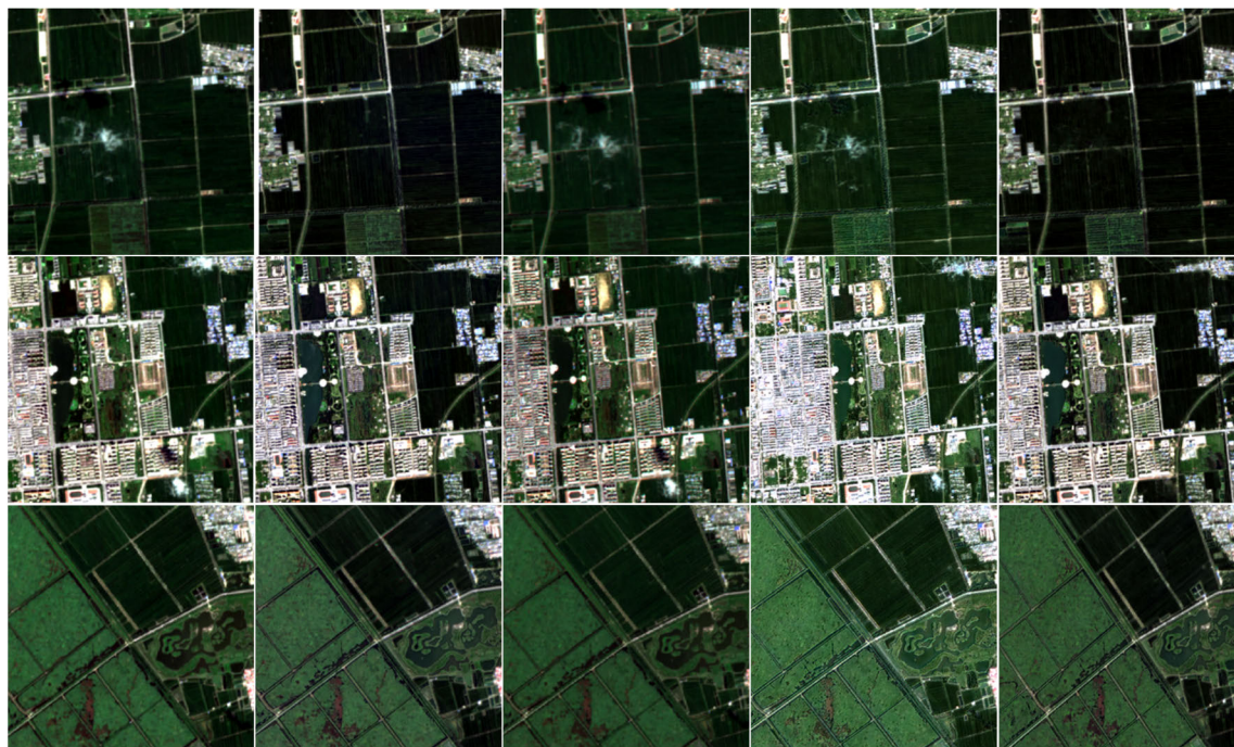
FIGURE 5. Comparison of SR results in large areas. From left to right: S2 original 10 m image, GF-1-pansharpened 2.5 m image, bicubic reconstructed sentinel-2 2.5 m image, SRGAN reconstructed sentinel-2 2.5 m image, and PGGAN-MSR reconstructed sentinel-2 2.5 m image.
