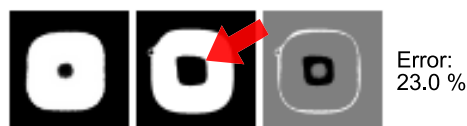
FIGURE 11. Dispense pattern involving a void area due to air entrapment. Left: output of ANN, center: experimental data with marked air entrapment, right: difference between ANN output and experimental data. Furthermore, we list the error score according to (2).
