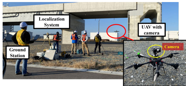
FIGURE 7. Our UAV inspection system uses a total-station-based localization system to enable UAV executing flight paths in GNSS-denied environments and collect photos.
