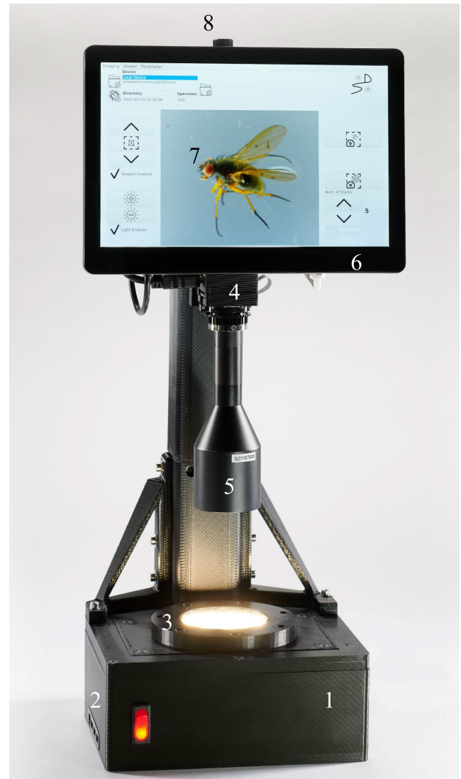
FIGURE 2. The standalone Entomoscope, with (1) base, (2) USB and network hub, (3) lighting, (4) 12 MP camera with (5) telecentric lens, (6) 10" HD touchscreen, (7) Graphical User Interface, and (8) manual focus wheel.
