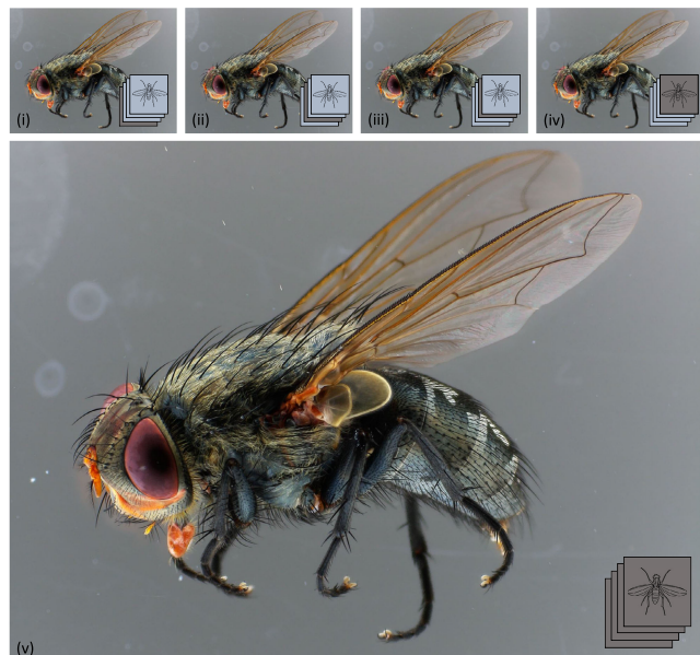
FIGURE 8. Single focal planes (i-iv) taken with the standalone Entomoscope for large-sized specimens (12 mm - 25 mm) and the fused image (v).
