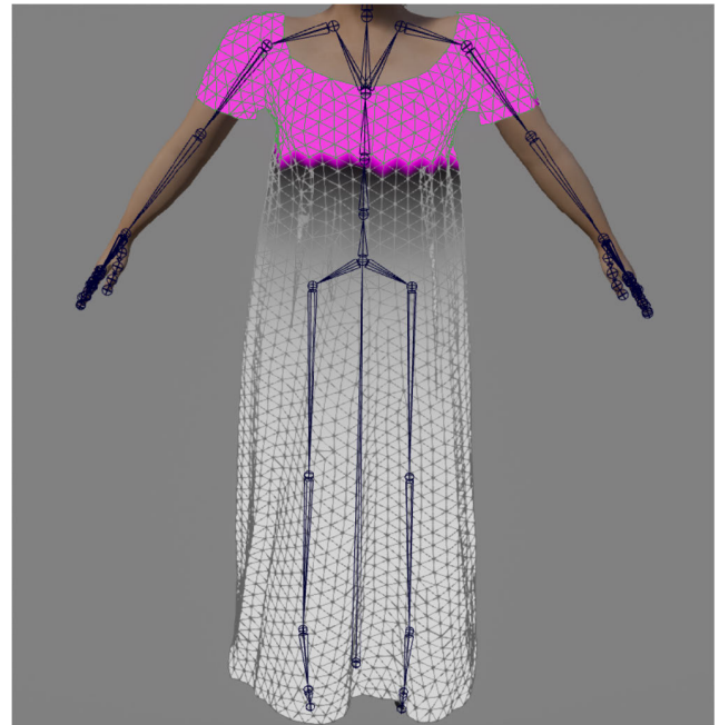
FIGURE 4. Proxy mesh example with skeleton and human upper body for reference. Proxy mesh parts controlled by skeletal animation are depicted in magenta, the physically simulated parts in the gradients of grey color.
