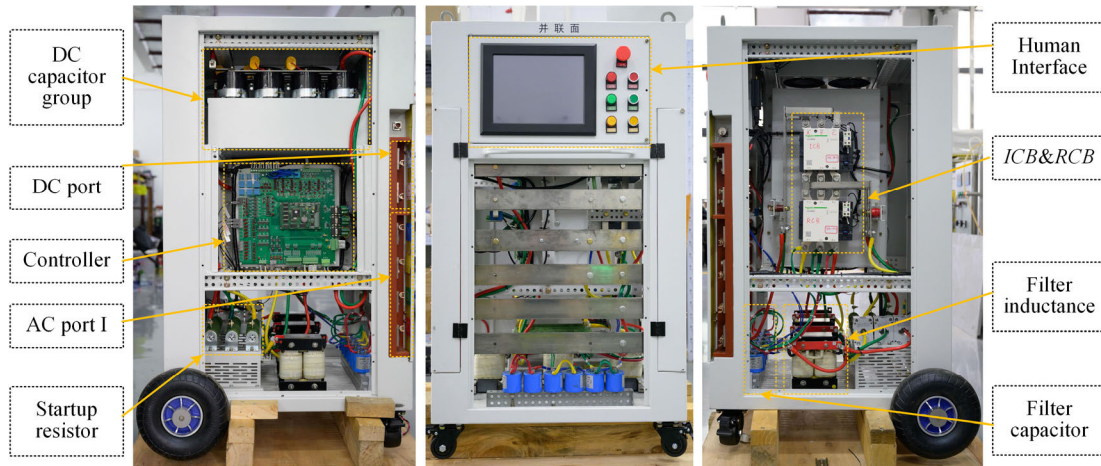
FIGURE 3. The mounting arrangement of the series inverter.
