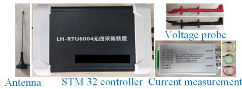
FIGURE 5. Components of remote measuring unit.
