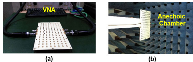
FIGURE 13. Measurement set-up for (a) S-parameters, and (b) radiation patterns and gain.
