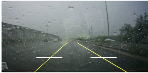
FIGURE 3. At 3/4 of the image, the detected lines were sampled along the white lines shown in the figure.
