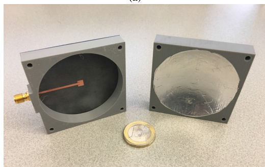
FIGURE 5. Compact parabolic reflector antenna: (a) schematic view and, (b) photography of the prototype (images extracted from [12]).
