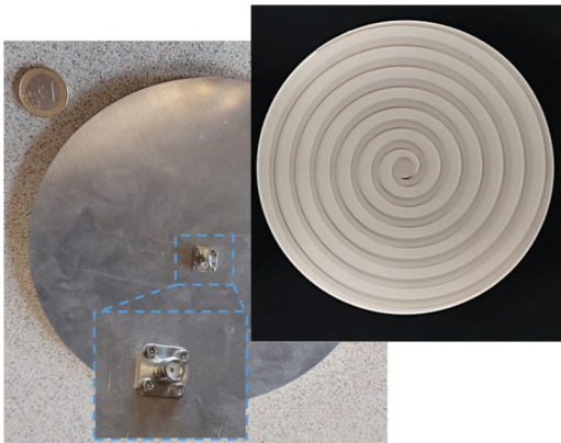
FIGURE 7. Bottom and top view of the 3D printed Archimedean spiral dielectric leaky wave antenna (images extracted from [14]).
