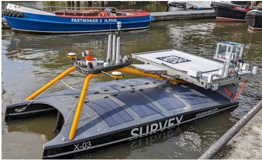
FIGURE 3. XOCAN vehicle (USV) with a battery hot Swap-system and landing pad - used during hamburg trials.
