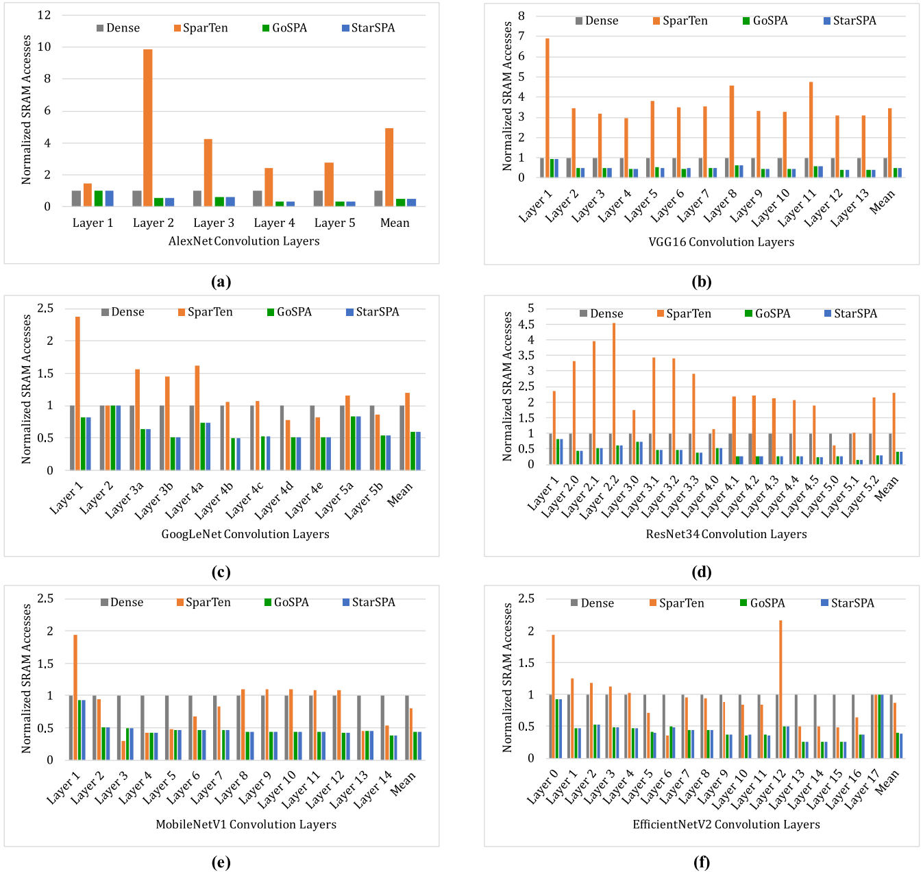
FIGURE 12. Comparisons on normalized SRAM accesses on convolution layers of (a) AlexNet, (b) VGG16, (c) GoogLeNet, (d) ResNet34, (e) MobileNetV1 and (f) EfficientNetV2 (baseline: Dense architecture).
