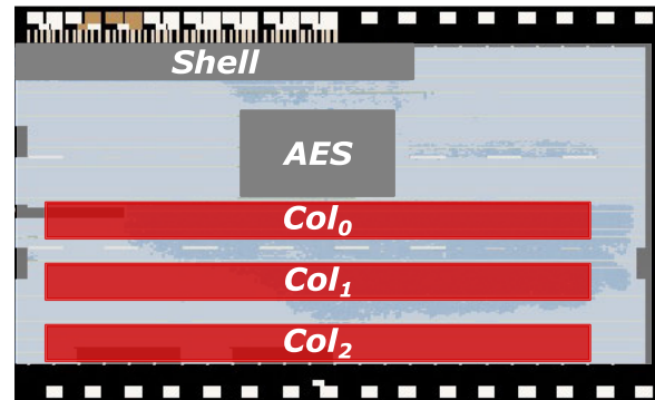
FIGURE 18. Floorplan for testing the effect of the distance on the success of X-Attack in the cloud. For space reasons, the view is rotated by 90°.
