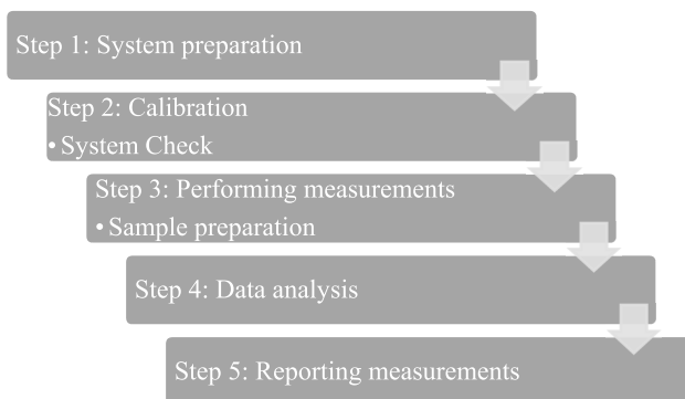
FIGURE 2. A block diagram breaking down the measurement process of complex permittivity in five main steps: system preparation, calibration, measurements, data analysis and final reporting of the measured data.
