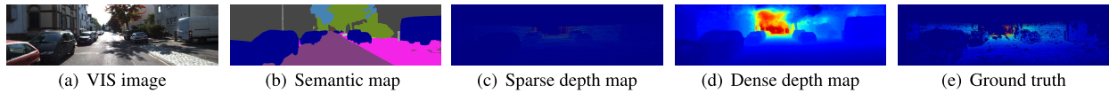
FIGURE 1. Examples of three different modalities: (a) VIS image, (b) semantic map, (c) sparse depth map, (d) predicted dense depth map, and (e) the corresponding ground truth.
