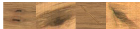
FIGURE 2. Common defects of wood floor such as dead-knots, live-knots, scratches and mildews.
