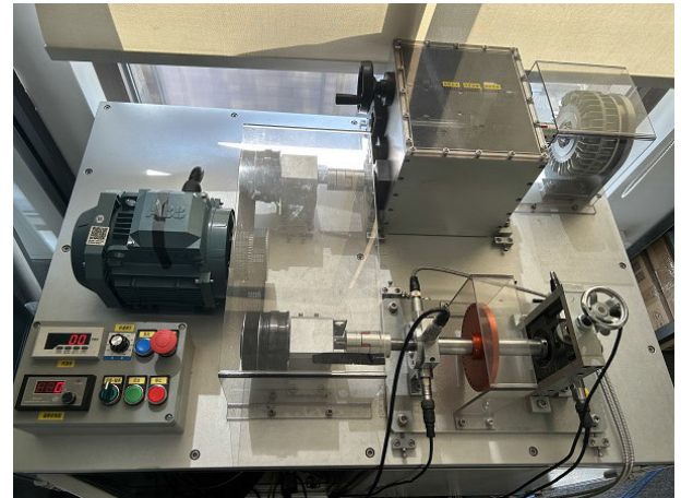
FIGURE 6. Multi-Speed rolling bearing data collection experiment equipment.
